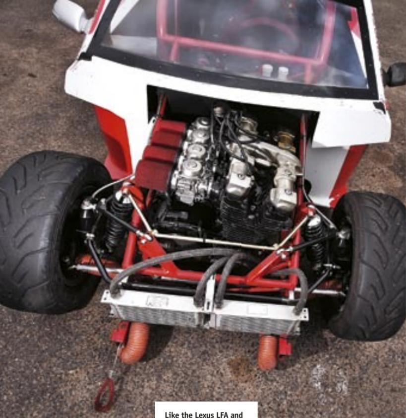
Like the Lexus LFA and IS-F, the Aussie Race Car Aurion has a Yamaha-developed engine too!
